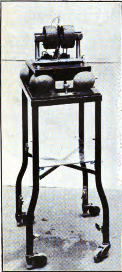
FIG. 64 a.—High-speed photographic receiver (galvanometer unit).
